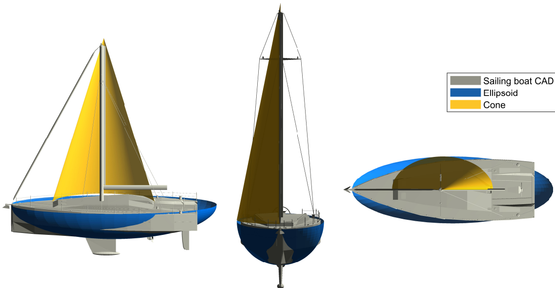
Figure 56: Sailing boat representation using a combination of a half-ellipsoid for the hull and a half-cone for the sail 6
