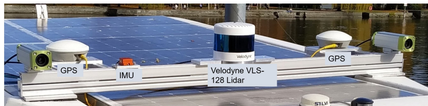
Figure 85: Sensor equipment: Velodyne VLS-128 lidar Alpha Prime, stereo cameras, GPS and IMU mounted on the research vessel Solgenia.
