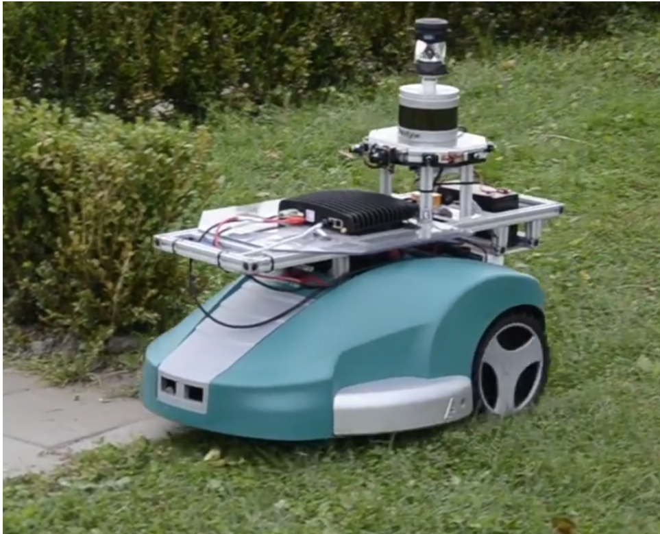
Figure 4.1: Motivating scenario: a prototype of a Bosch autonomous lawn mower equipped with a LiDAR. Image courtesy of the Trimbot project [111].
