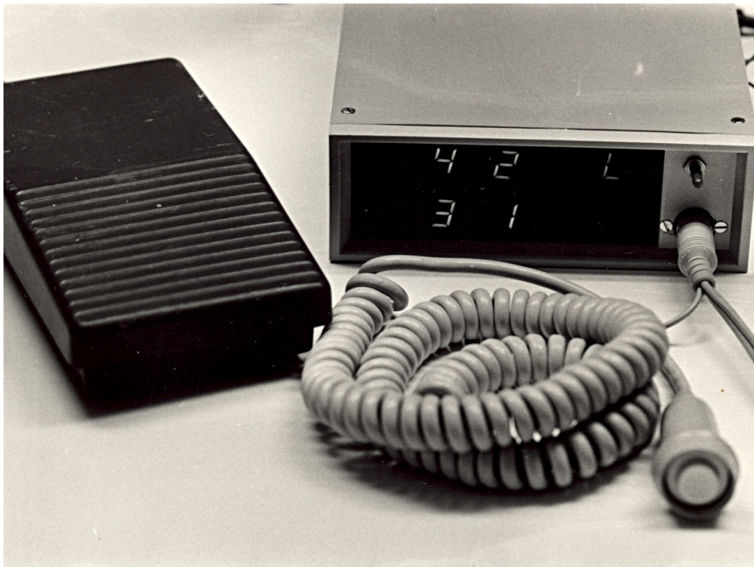
Fig. 5 Selfmade electronic counter 16 with foot and hand switches
