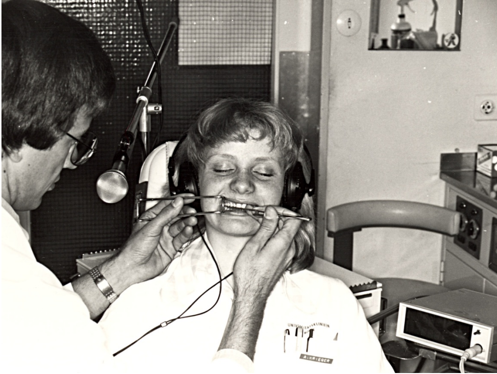
Fig. 3 Test setup for determining tactile sensitivity using copper foils.
