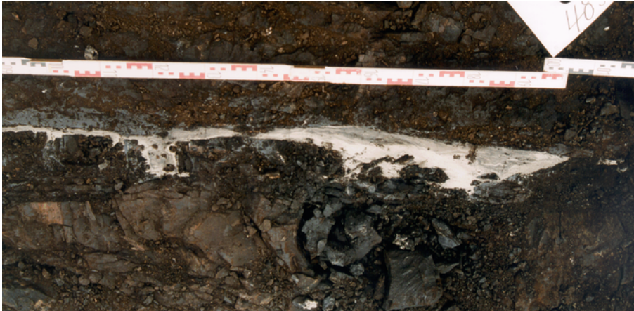
Fig. 2.8: Horizontal section of a fault gouge in lignite that solely contains white clay smear (picture width: 1.20 m).
