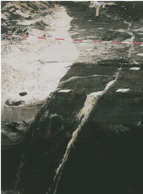
Fig. 3.10: Horse structure at the branching zone of main fault (white shear band to the right) and splay fault (shear band between white sand and dark lignite to the left). – Lower part of the picture is a vertical section; upper part is a horizontal section. Picture width: approx. 3.5 m
