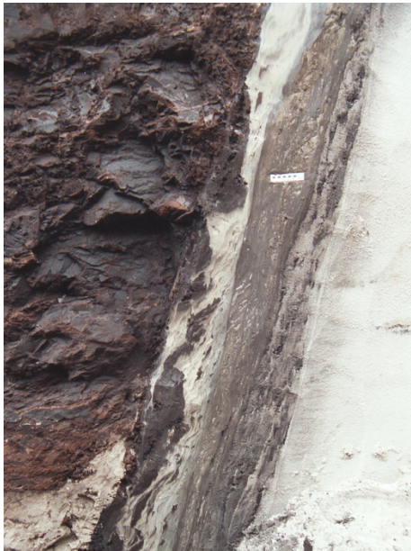
Fig. 2.4: Vertical cross section of a shear zone showing all lithologies that have been found in the fault gouges. Width: 25 cm. A: sand (footwall), B: lignite (hanging wall), C: clay layer, a: sand with bituminous clay (dark), b: dark clay and sand, c: white clay, d: bituminous clay, e: lignite fragments.
