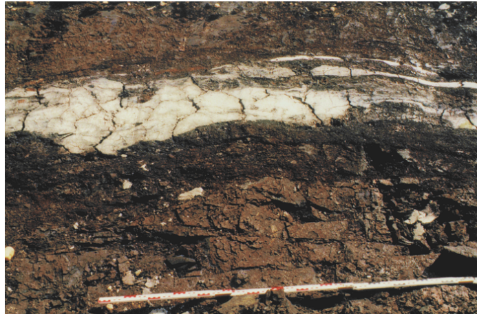
Fig. 2.6: Intense fragmentation of lignite adjacent to the clay smear (horizontal section; picture height: 1.24 m).
