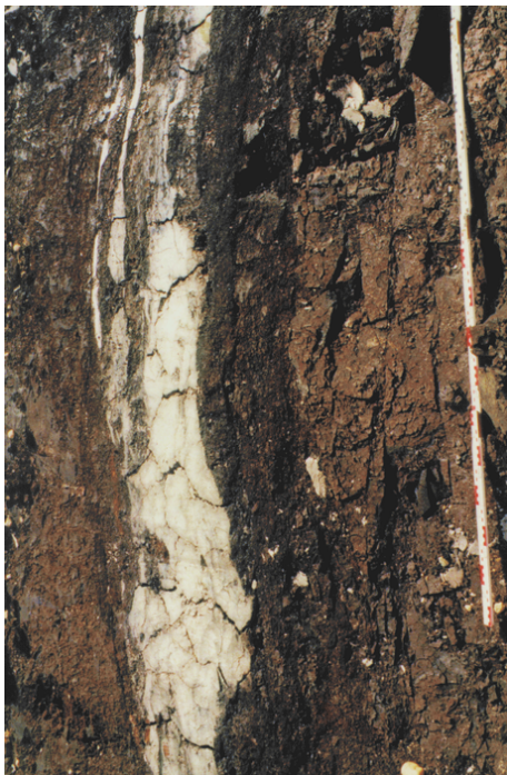
Fig. 3.13: Horizontal section showing damaged lignite adjacent to the white clay smear (left side is foot wall).
