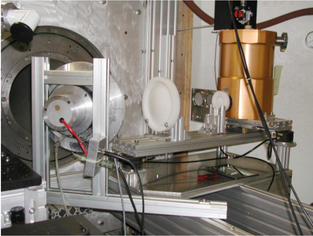
Figure 5.16: PolKa at the HHT on January 2002. The 246 mm RHWP is seen from the back, on its left is the Nasmyth tube, on the right are the lenses and the receiver. See also figure 5.2
