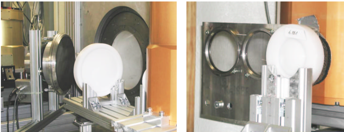
Figure 5.17: Left : PolKa as seen from the receiver. In the background is the HEB receiver. Right : A detail of the frame holding the two analyzers.
