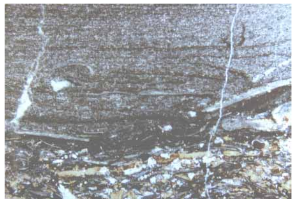
F: Biowackestone microfacies. Sample AR 9 from the Sundance Formation at section Alcova Reservoir (scale is 1,1 cm for the long side of the photo). Densely packed pelecypod fragments grade upward into convolute laminated fine-grained sandstones.
