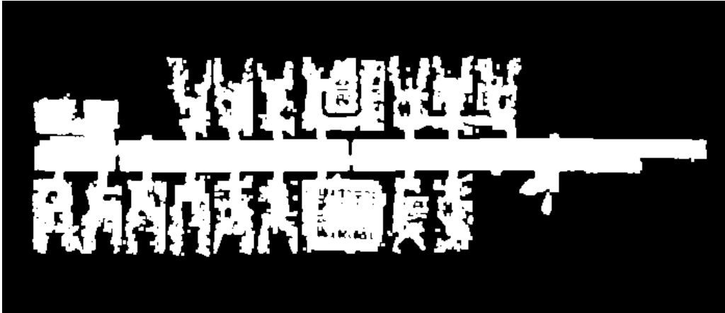
Figure 2.5: A learned occupancy grid of the first floor of the Department of Computer Science III at the University of Bonn. It has been learned by the mobile robot RHINO using two laser range finders.
