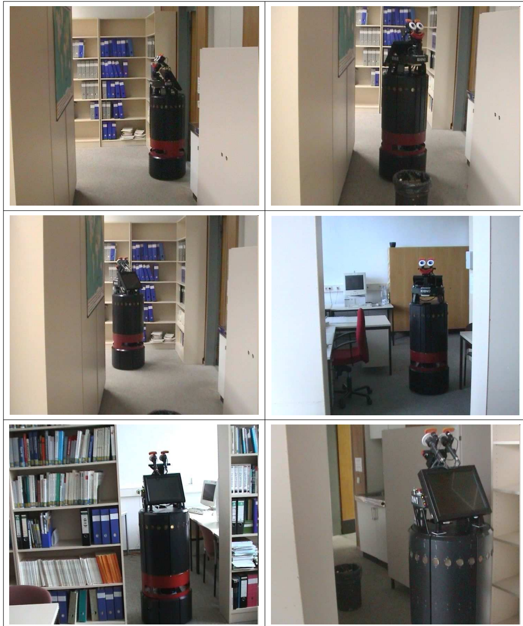
Figure 4.11: The mobile robot RHINO performing replanning when confronted with an unexpected obstacle.
