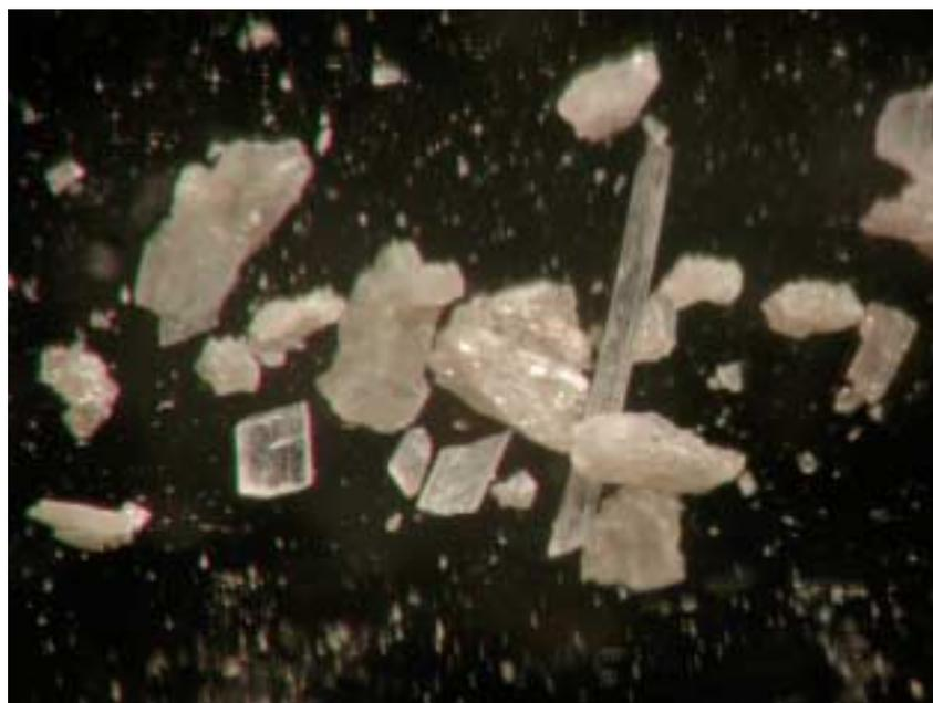
**Abb. 9.1:** Kristalle von (Bi<sub>2</sub>Cl<sub>4</sub>)[AlCl<sub>4</sub>]<sub>2</sub>.
