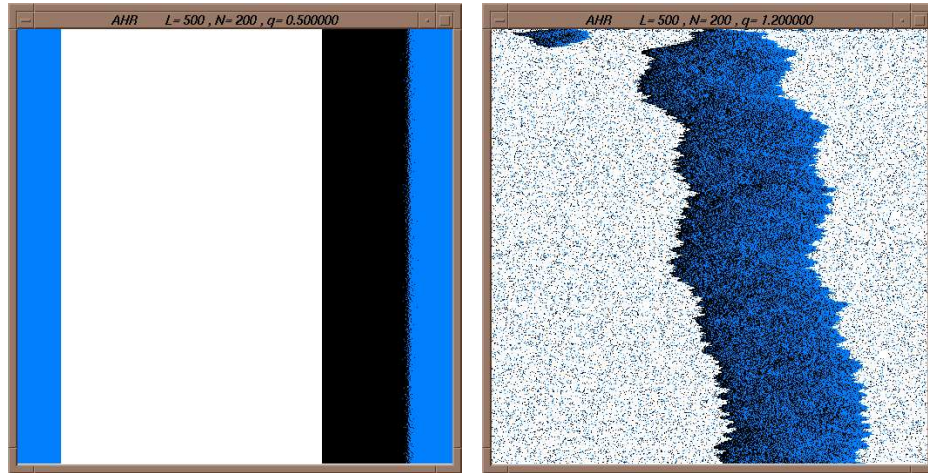
Figure 2.1: Left: Strongly phase separated phase of the AHR model at q = 0.5 . The system has a length of L = 500 with 100 particles of each species. Vacancies are white, + particles black and - particles grey. Time is running top-down, space from left to right. Right: Disordered phase of the AHR model at q = 1.2 . Due to the large correlation length the system appears to be softly phase separated.
