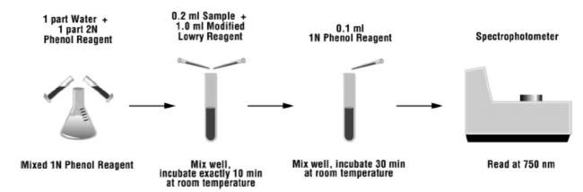
Figure V/1.1: Test tube procedure (Lowry's method) 391
