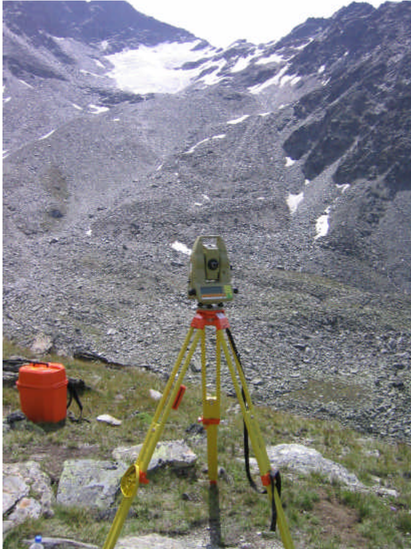
Figure 3.7: Total-station on one of the reference points situated on a latepleistocene moraine with an overview of the research object (rockglacier in the background).
