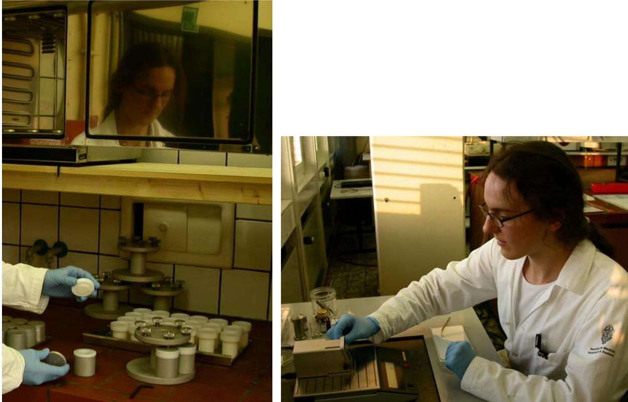
Figure 16: Preparation of wet acid digestion with nitric acid (left) and weighing of samples for elemental N analysis (right)
