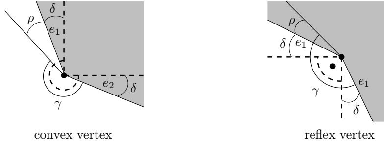
Figure 3.9: Maximal deviation between the outer measured angle ( \gamma ) and the outer nominal value (dashed) for a convex and a reflex vertex.
