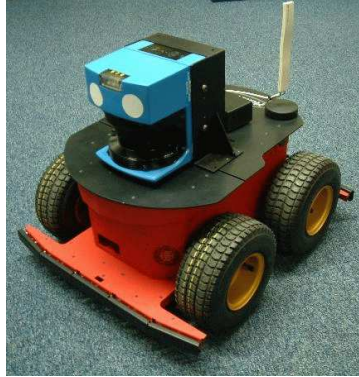
Figure 1.1: A mobile robot (Activmedia Pioneer P2-AT) equipped with a laser scanner (Sick).
