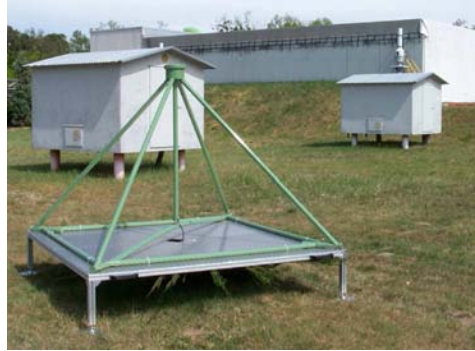
Figure 2.2: One of the LOPES antennas at the KASCADE-Grande site. The active balun resides inside the container at the top of the antenna. The radiator consists of cables in two opposing edges of the pyramid. By choosing the east-west edges our antenna is sensitive to the east-west polarised component of the radiation.
