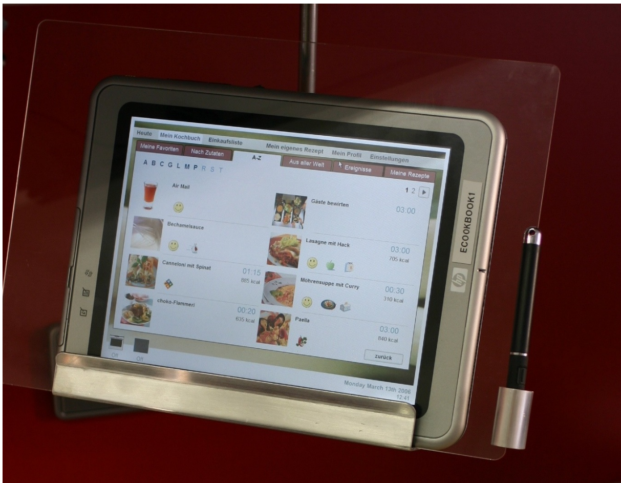
Figure 3-1: The electronic cookbook prototype in its stand, with plexiglass cover.
