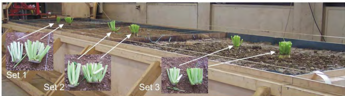
Figure 6.34 Scenario with sugar beets with leaves' brush; a) with long brushes (ca. 40 cm), b) with short brushes (ca. 20 cm)
