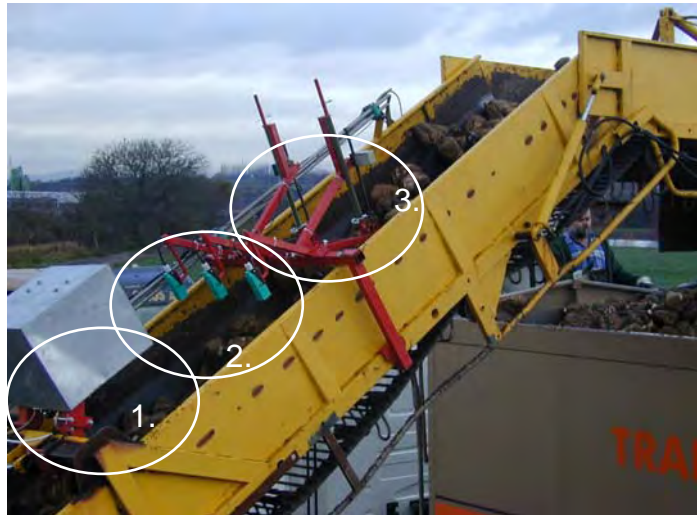
Figure 2.1 Positions of the indirect sugar beet yield recording systems on the elevator: 1. laser system, 2. ultrasonic system, 3. mechanical finger-sensing system (Schmittmann et al. 2001)
