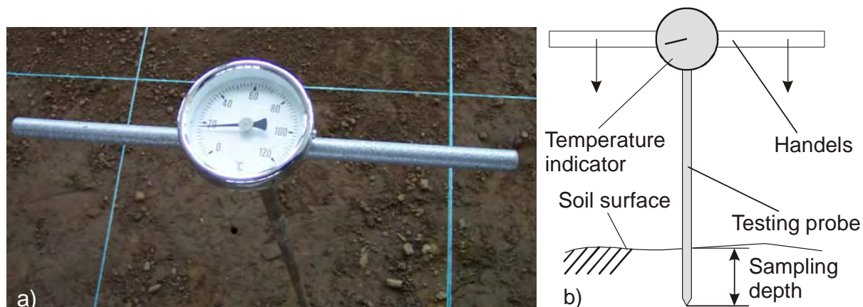
Figure 6.14 Soil temperature sampling probe; a) probe in the soil, b) main parts of the probe and sampling principle
