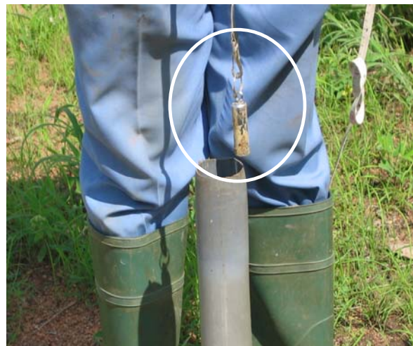
Figure 5.8: Bell tape measurer for monitoring the water levels inside the piezometer
