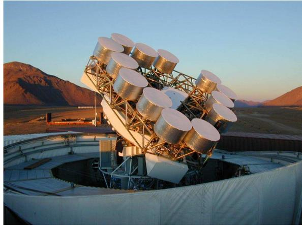
**Figure 1.5:** The Cosmic Background Imager (CBI) at its open configuration for observing with high angular resolution. This mode is for total intensity measurements.
