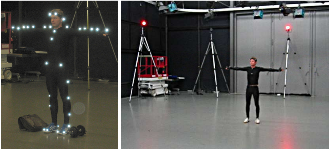
Figure 1.3. Passive optical motion capture system based on retro-reflective markers attached to the actor’s body. The markers are tracked by an array of six to twelve calibrated high-resolution cameras arranged in a circle around the capture volume, which has a radius of approx. 2.5 m in this example.
