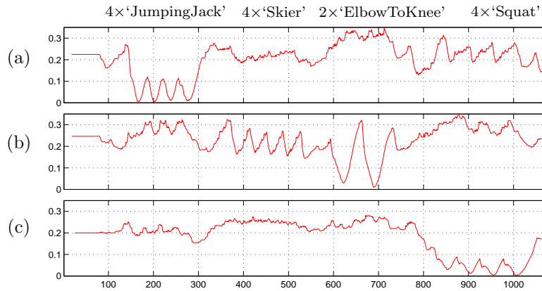
Figure 5.7. Resulting distance functions for a 35-second gymnastics sequence (30 Hz) consisting of four jumping jacks, four repetitions of a skiing coordination exercise, two repetitions of an alternating elbow-to-knee motion, and four squats with respect to the quantized class MTs for (a) ‘JumpingJack’, (b) ‘ElbowToKnee’, and (c) ‘Squat’.
