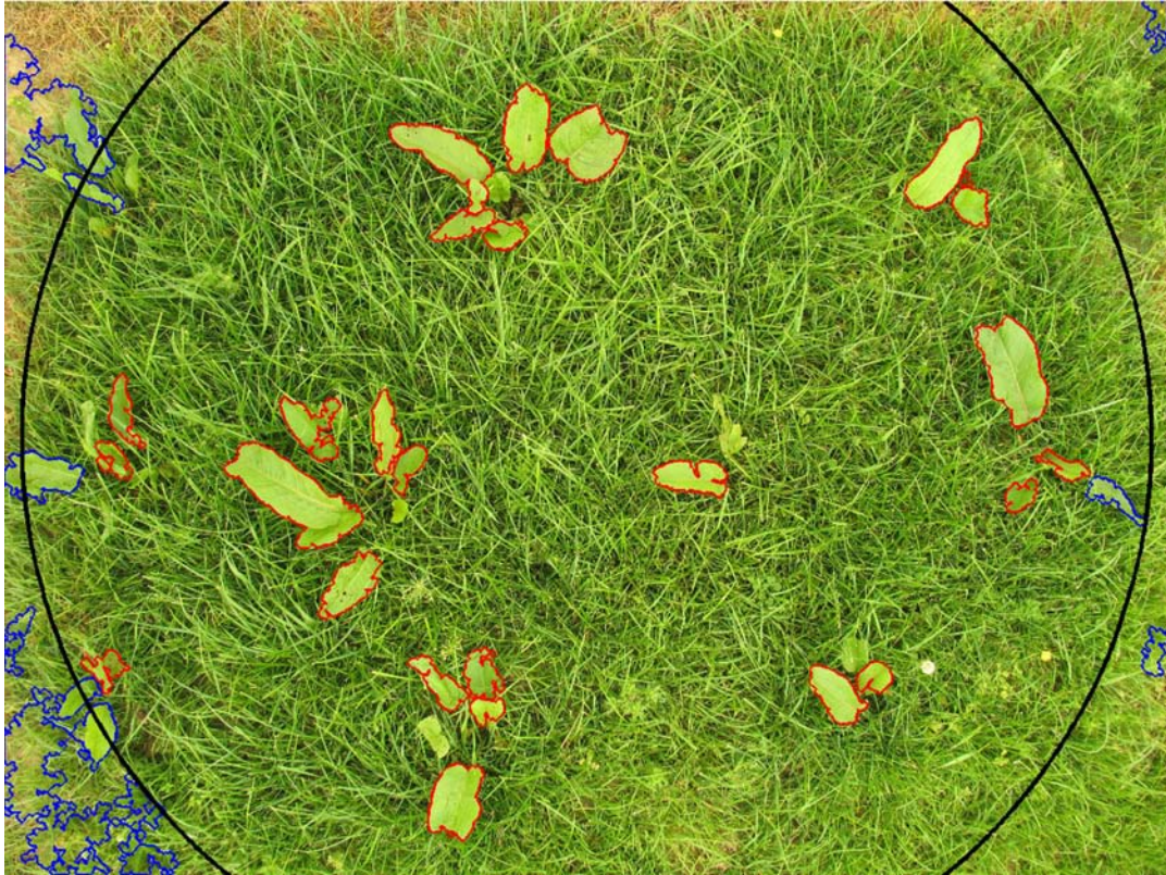
Figure 4.1.: Confidence circle CC: only the red objects lying completely within the black circle are included in the classification
