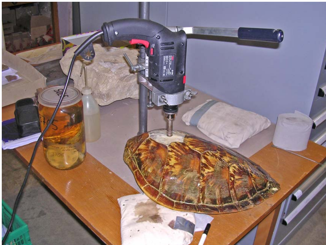
Figure 6: Sampling of the turtle shell by core-drilling. The cores (12 and 22 mm in diameter) are taken with diamond-sintered hollow drill bits and a standard power drill with adjustable drilling speed mounted on a drill press.
