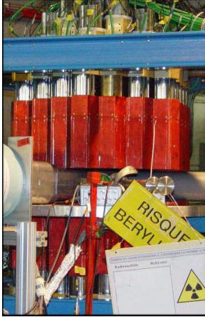
Figure 3.4.: The Château de Cristal is built of 74 \text{BaF}_2 detector crystals embedded in red aluminum cans. The PMTs extend beyond these cans. The name crystal castle is due to the geometry with all detectors aligned perpendicular to the beam plane.
