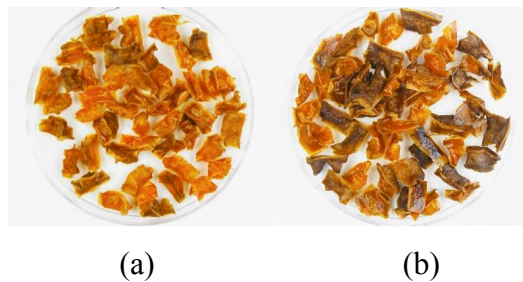
Fig. 6.11: Visual comparison of tomato samples dried intermittently (a) and continuously (b) at 150 °C
