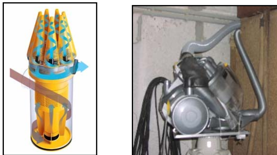
Figure 3.26: Vacuum cleaner working with root cyclone technology system (left: working theory, right the used cyclone)
