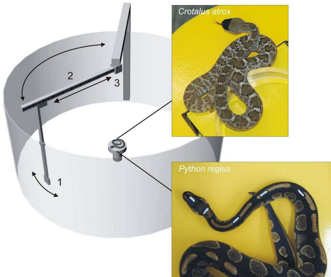
Fig. 4: Schematic sketch of the experimental set-up. 1: IR source (PE), 2: scale (100 cm), 3: video camera (not shown). Arrows indicate the moving directions of the IR source. Insets show representatives of the two snake species C. atrox and P. regius , both blindfolded.
