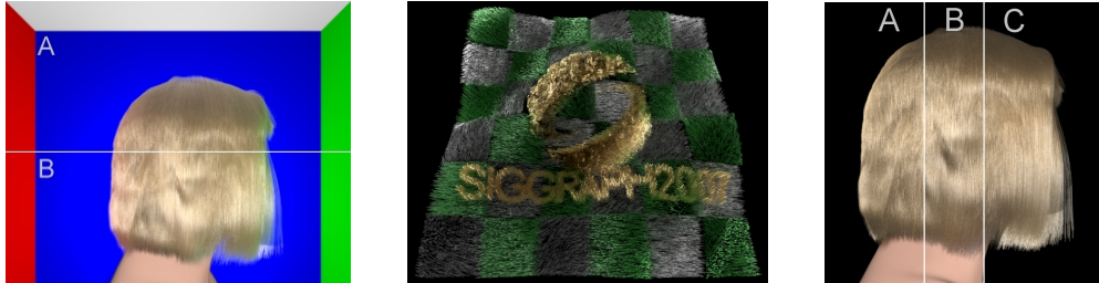
Fig. 4.14: Left: Color Bleeding. Split-screen comparison of our ray-based approximation, which is used for rendering the lower half of a blond hair style (B), with a path tracing reference used for the upper part (A). Middle: A carpet made of a mixture of fibers including the SIGGRAPH logo in golden fibers rendered with our ray-based approximation method. Right: Comparison: “double scattering” approximation (A, cf. Sec. 4.10), a path tracing reference (B), and our ray-based approximation (C).
