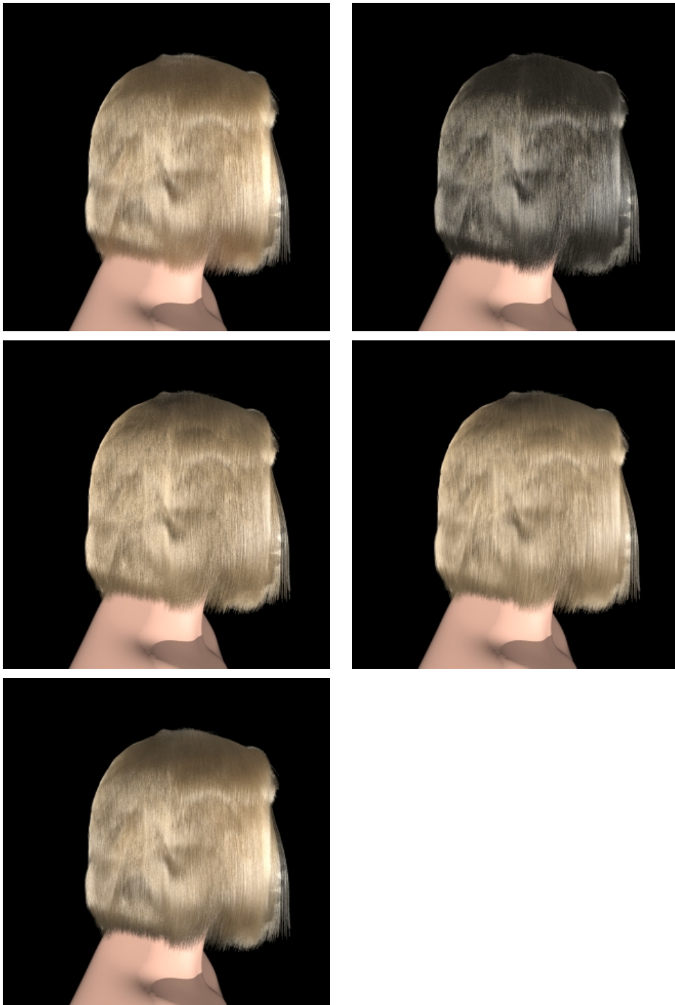
Fig. 4.26: A blond hairstyle illuminated with four directional light sources. Comparison of results obtained with: path tracing (reference) (top left), ray-based global illumination (bottom left), “double scattering” approximation using maps (middle right), “double scattering” approximation with ray shooting (middle left), single scattering only (top right).
