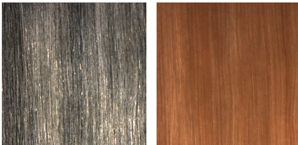
Fig. 4.6: Measurements of blond hair using the method of [45] (images from http://www1.cs.columbia.edu/CAVE/projects/separation/separation_gallery.php ) Left: single scattering, Right: multiple fiber scattering. Note the smooth and even scattering distribution of multiple fiber scattering and the sharp azimuthal details of single scattering.
