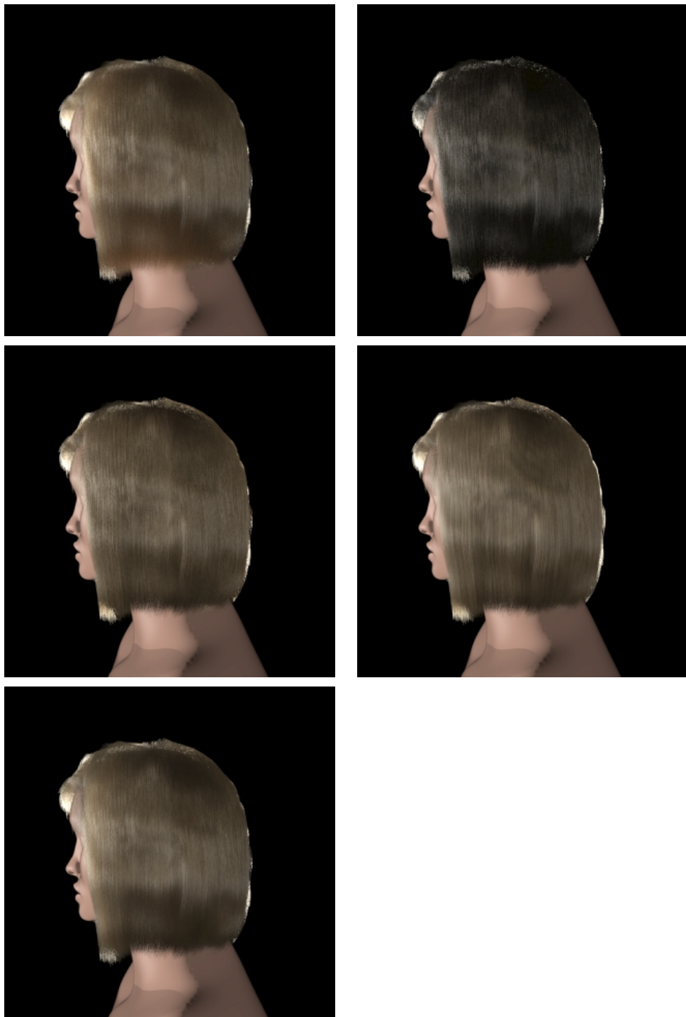
Fig. 4.27: A blond hairstyle illuminated with four directional light sources. Comparison of results obtained with: path tracing (reference) (top left), ray-based global illumination (bottom left), “double scattering” approximation using maps (middle right), “double scattering” approximation with ray shooting (middle left), single scattering only (top right).
