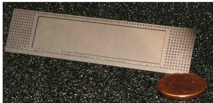
Figure 2.15: Cross section and photograph of a mockup module with thinned 'sensitive area' and a thicker silicon support frame. The readout and steering chips are directly bump-bonded onto the Si-support frame.
