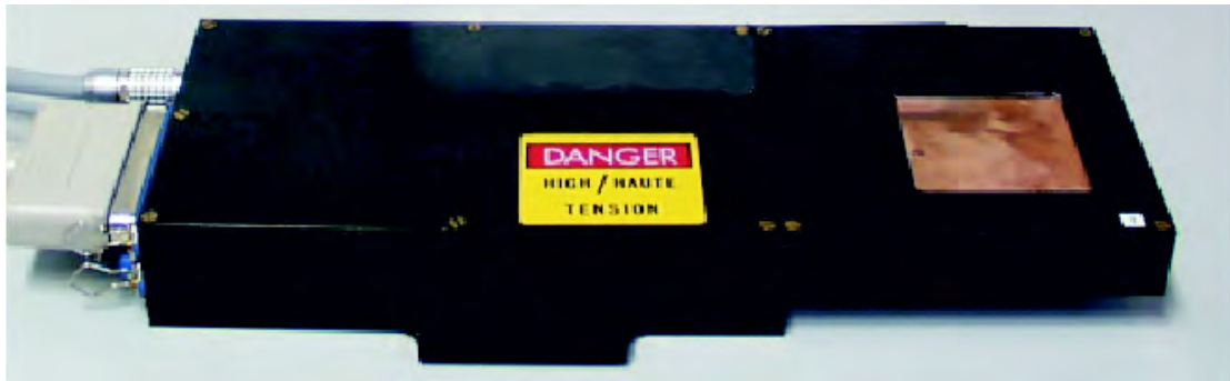
Figure 6.4: Picture of a Bonn Atlas Telescope Module (BAT) [53]
