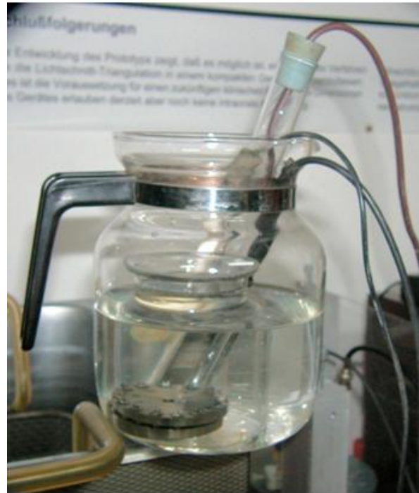
Figure 13. Aging of the specimens in a pot of 37°C distilled water containing an aquarium heating device and an electronic thermometer.
