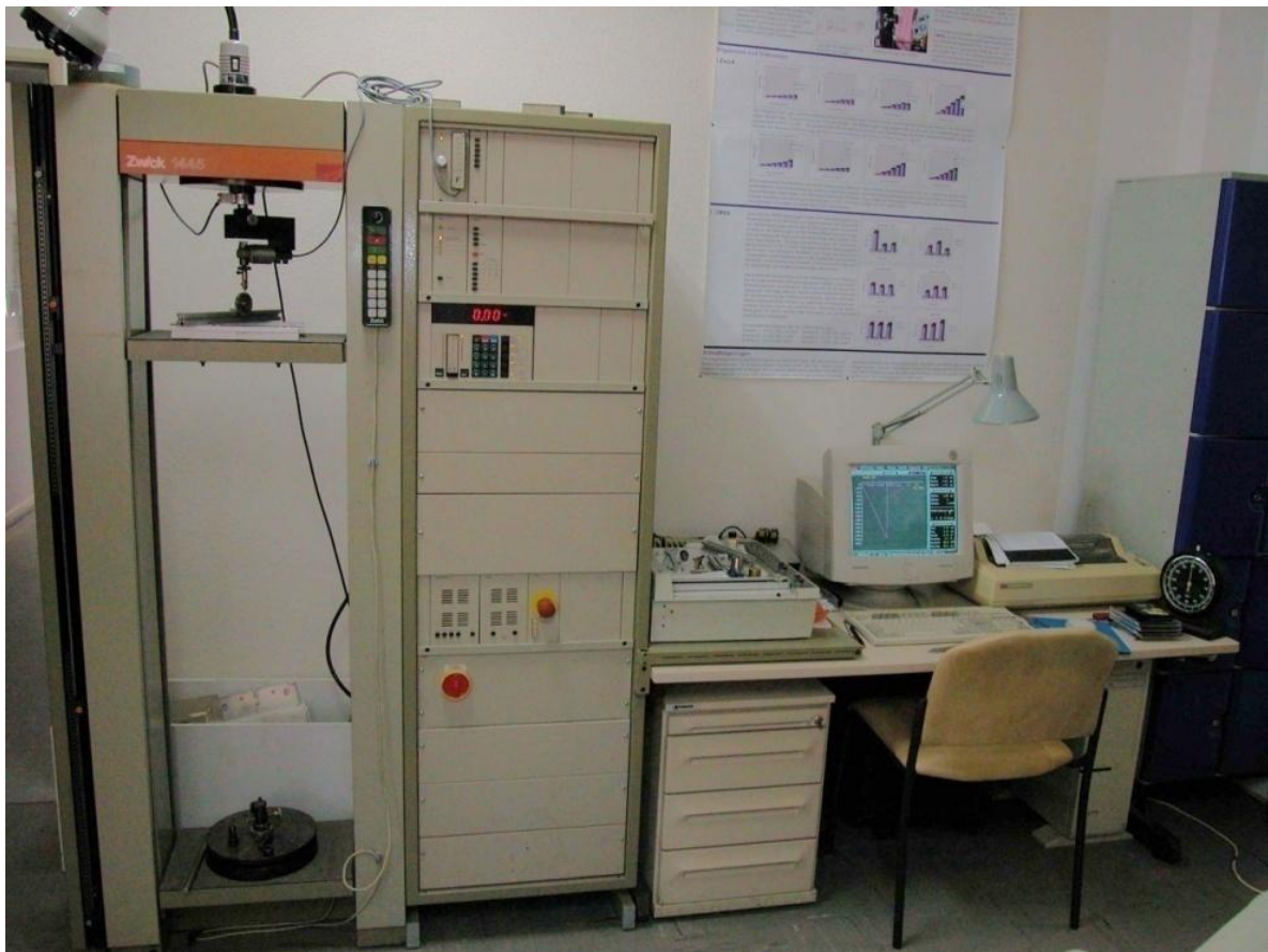
Figure 14. The universal testing machine Zwick 1445.
