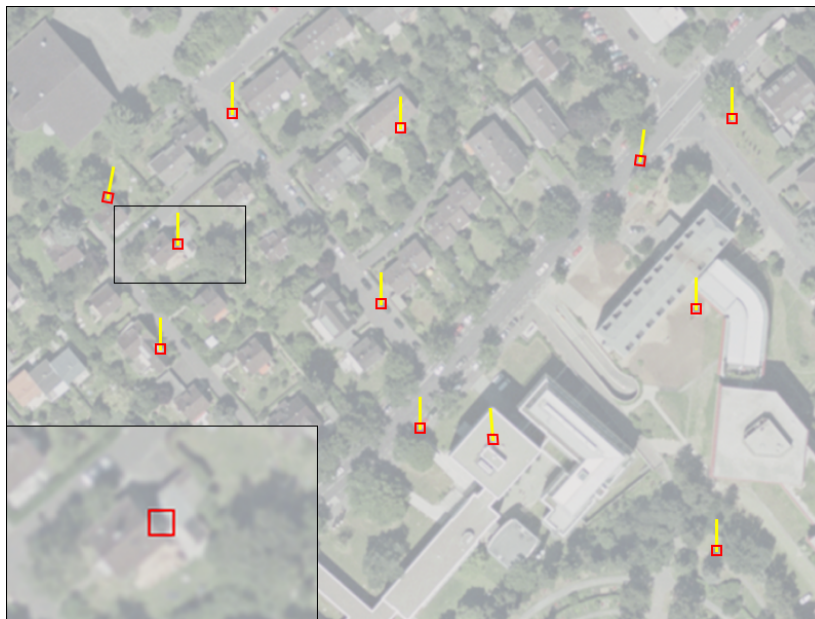
Figure 4.2: Example for point based feature tracking assuming small disparities in consecutive frames. The red box marks an extracted feature, the yellow line is the displacement vector of the feature to the consecutive image. In the lower left corner a detail of the image is enlarged.
