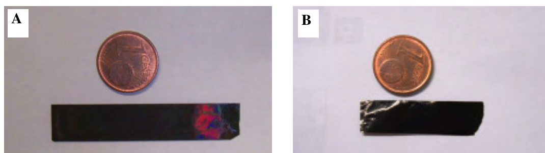
Figure 5.17: Digital camera pictures of a CNT-based film created on a polystyrene mask (A) and its free-standing form obtained after chemical delamination (B).
