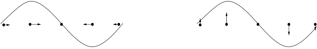
Figure 2.1: An example of longitudinal (left) and transversal (right) waves of a 1d chain in 2d. The arrows show the displacement direction of the particles
