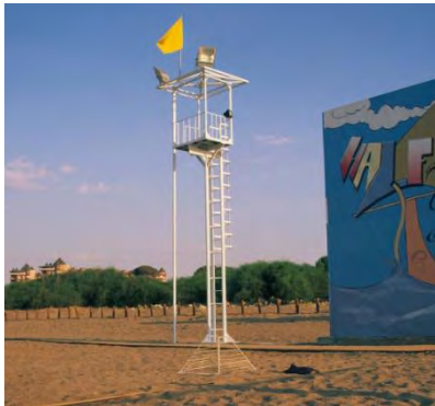
Figure 4.14: MH light in close proximity to a protected sea turtle nest (Section II). Mounting height: 8 m
