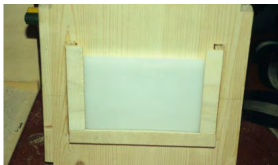
Figure 5.7 b: Acrylic glass placed in front of the Halogen lamp, for reducing illuminance in the box
