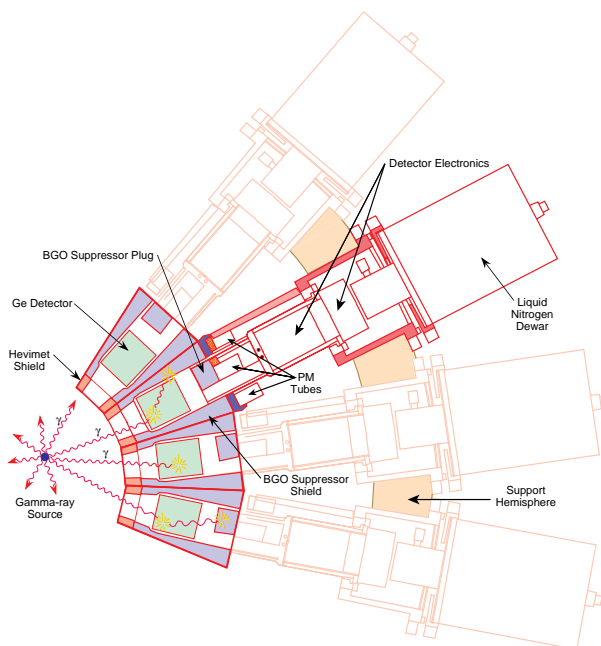
Figure 3.5: Schematic illustration of Ge detectors with Compton-suppression shields.
