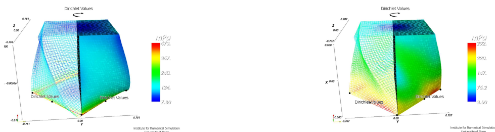
Figure 6.2: Application of INTERPRETLIB for Boundary Values. Here, we describe displacements by means of the coordinates at the respective quadrature points, yielding a rotation of the upper plane of about 45^\circ . The left image shows the result for linear elasticity, the right image for an Ogden material, as employed in Chapter 5.5.
