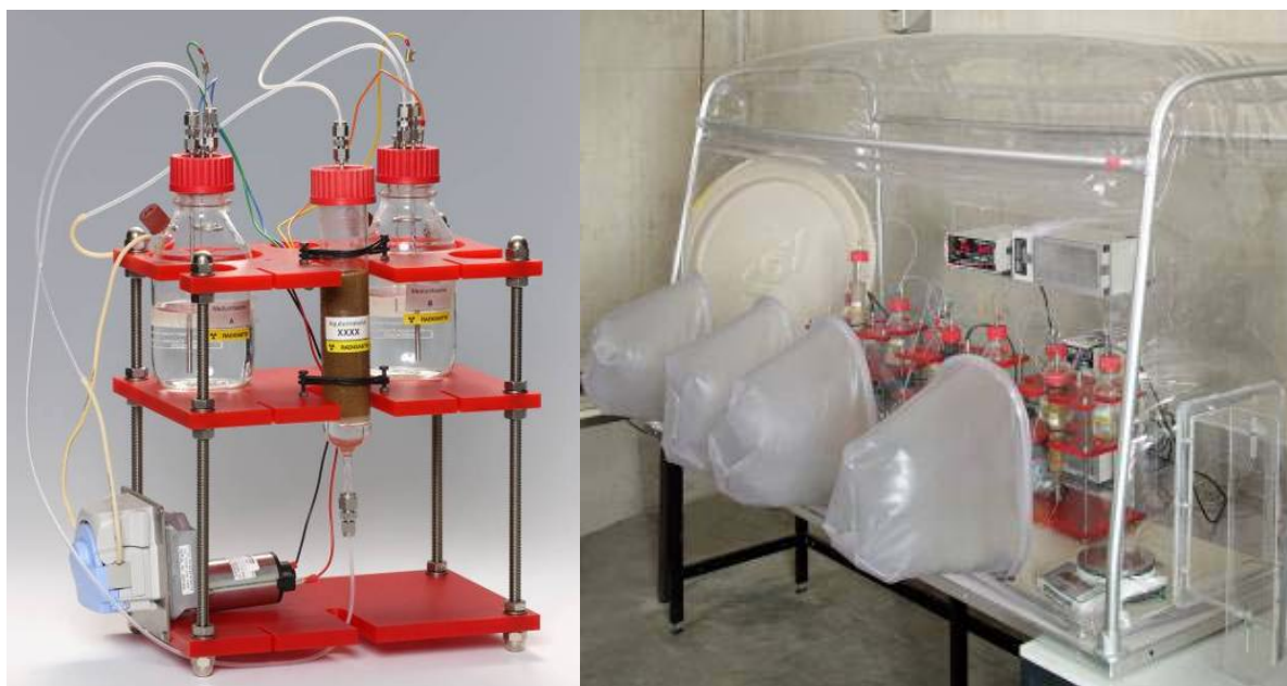
Figure 12: The DAISY incubation test system: Design and experimental setup inside an atmospheric chamber
