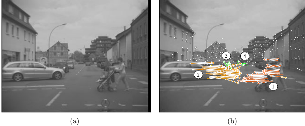
Figure 3.15.: 6D-Vision results of a scene with four moving objects: (1) A pedestrian with a stroller walking to the left, (2) A vehicle turning into the street from the left, (3) A slow oncoming vehicle, and (4) a vehicle moving from left to right at a far distance. The arrows indicate the predicted linear point motion for the next half a second. Clustering of neighboring 6D vectors with common motion yields object candidates.
