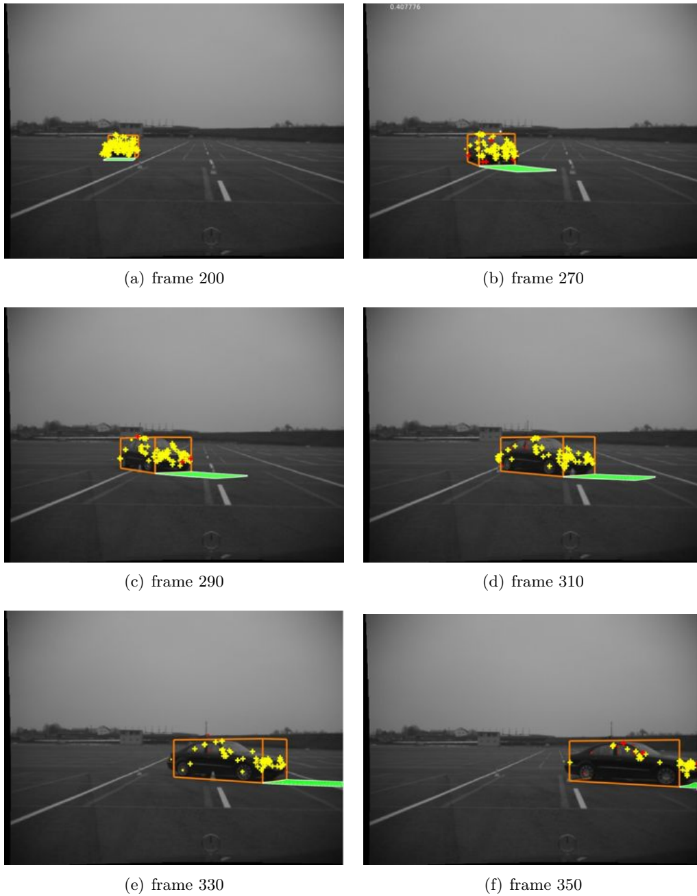
Figure 4.19.: Scenario 1 from the perspective of the ego-vehicle. The tracking results are superimposed. The bounding box indicates that the system is able to reconstruct the object pose very precisely during the maneuver.
