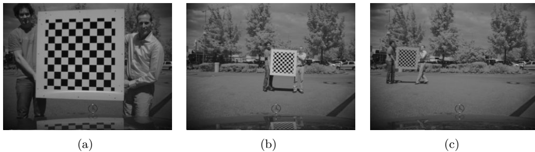
Figure 2.3.: Example images used for calibrating the intrinsic and extrinsic parameters of the stereo system. The checkerboard is captured at several poses and distances all over the viewing field of the cameras.
