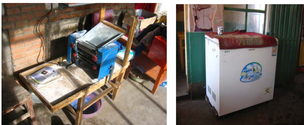
Photograph 4-4 High-power electrical appliances, 500W noodle machine (left) and 2200W freezer (right), in Saierlong Township
