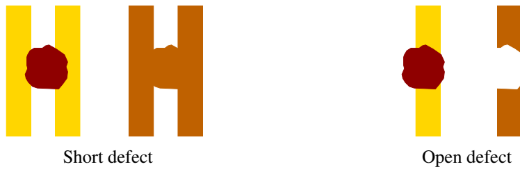
Figure 4.2: Short (extra material) and open (missing material) defects, and resulting damages to the chip layout (“faults”)
