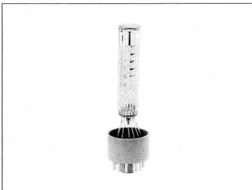
The BURLE 83087 100 is a 19mm (3/4-in) diameter end-window PMT with a 10-stage linear focused alkali-antimonide dynode structure, bialkali photo-cathode, and semiflexible leads to which a 12-pin base is soldered. The PMT features high QE (typically 27% at 370nm), high gain and compact size. It is well suited for photon counting, positron emission tomography (PET) scanners, and other scintillation detection applications such as electron microscopy, fluorescence spectroscopy, pollution monitoring.
