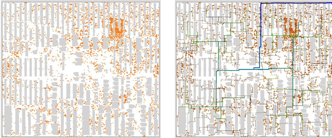
Figure 3.1: A clock tree instance and a complete clock tree. The sinks are in orange, the source is placed in the upper right corner. The color and thickness of the wires in the right picture depend on the arrival time of the clock signal (blue and thick is early, red and thin is late).
