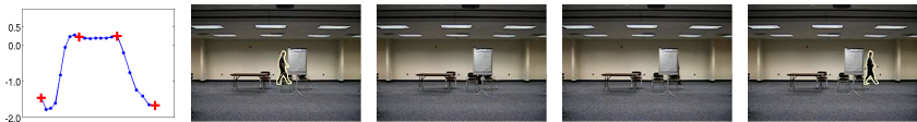
Figure 2.9: Detection of inconsistent solutions. The plot on the left shows the image energy E_{TV} as a function of the frame number. Red crosses indicate the four frames shown on the right. Incorrect segmentation results due to a total occlusion of the object of interest can be automatically identified and suppressed (2nd and 3rd frame).
