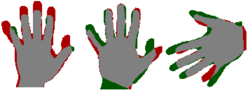
Figure 3.9: Region based distance. The region based distance is looking for a rotation and translation such that the area of the symmetric difference is minimized. This symmetric difference consists of the following two components. The first one (green) represents the region of the first shape that is not a part of the second shape. The second component (red) is the region of the second shape that is not part of the first shape
