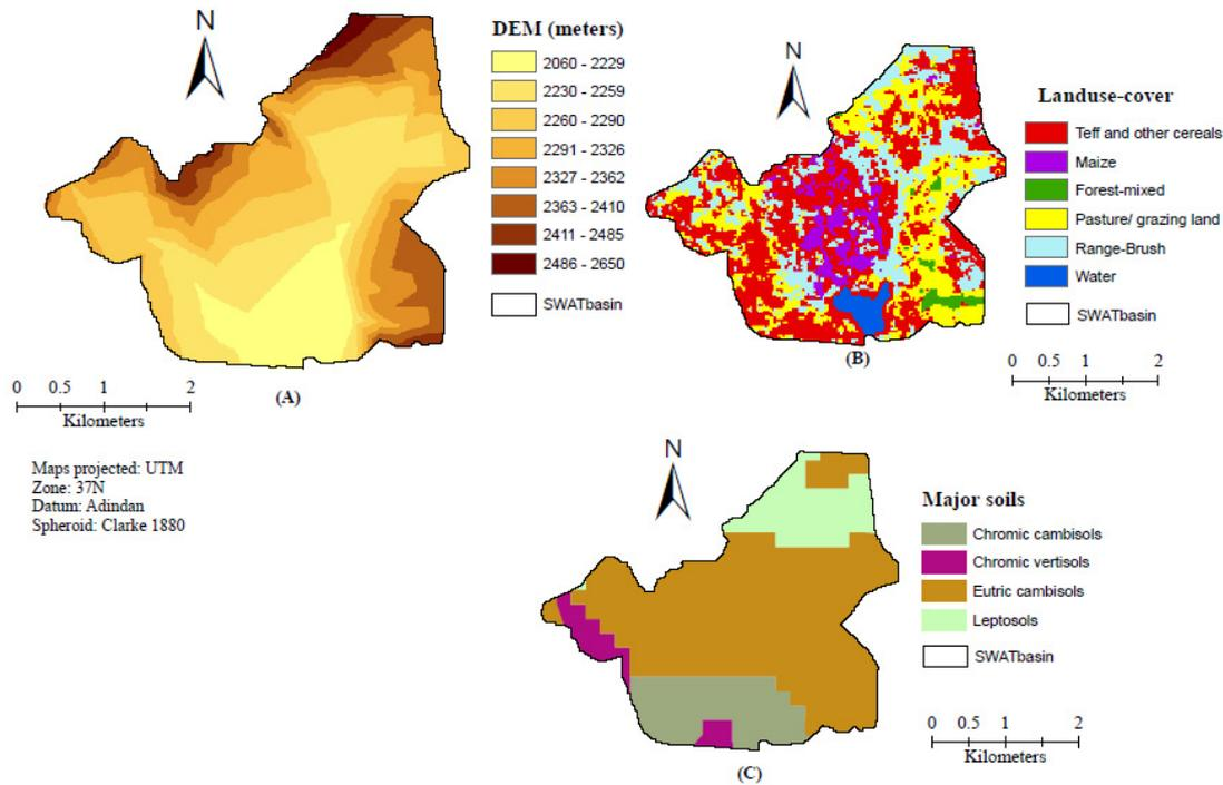
Figure 7.2: SWAT model inputs: (A) Digital elevation model (DEM), (B) land-use and land-cover and (C) major soils of Mai-Negus catchment, northern Ethiopia
