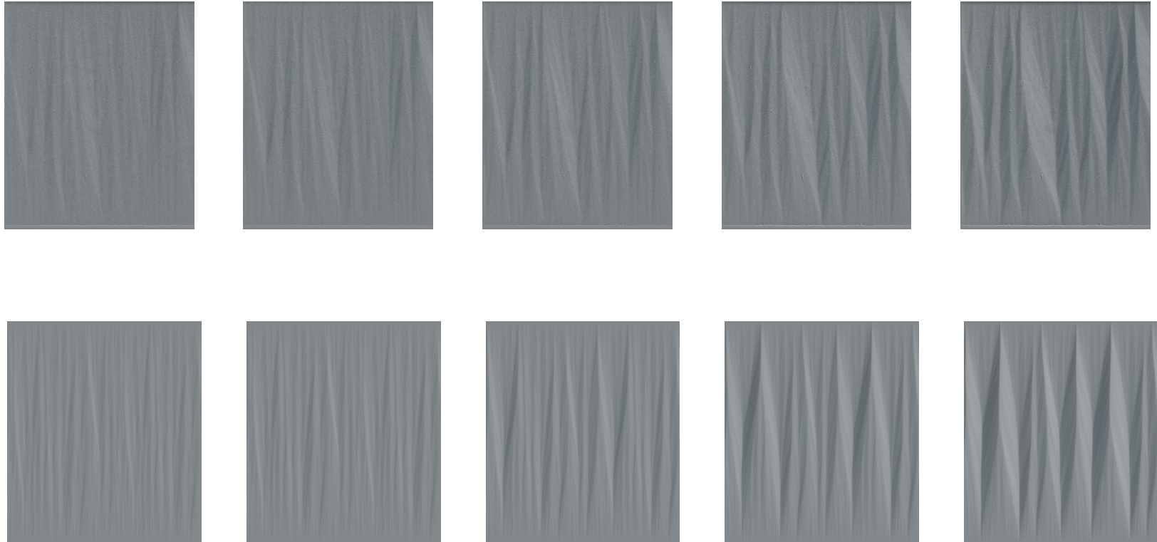
Figure 1.30.: Experiment and numerical simulations: The coarsening of the concertina pattern in a Permalloy sample (top row) of 30 nm thickness and 70\ \mu\text{m} width compared to the numerical simulations (bottom row). A ripple-like structure grows into the concertina pattern. Within the numerical simulations we iteratively increment the external field and minimize the energy, see Section 4.7. The computational domain is of period 6\hat{w}^* . The numerical images are scaled according to (1.11). The images hence display approximately 1.8 times the unit cell; the numerical images therefore appear to be more uniform than the experimental concertina. Details on the numerical simulation of the random anisotropy are discussed in Subsection 7.1.2.
