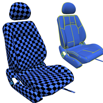
Figure 8.1: A CAD model with non-manifold edges and gaps (marked yellow). Our method can create texture maps for such inconsistent triangulations that are smooth at gaps and boundaries.
