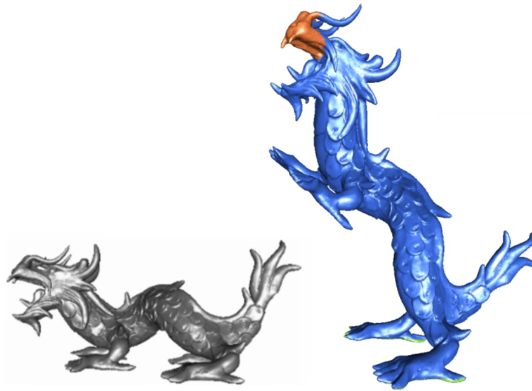
Figure 1.2: Original shape and result of an interactive editing session. The result was obtained by fixing parts of the dragons back feet (shown in green) and pulling parts of its nose (shown in orange) upward. The surface deformation interpolates the transformation of the nose over the surface but preserves shape details as much as possible.
