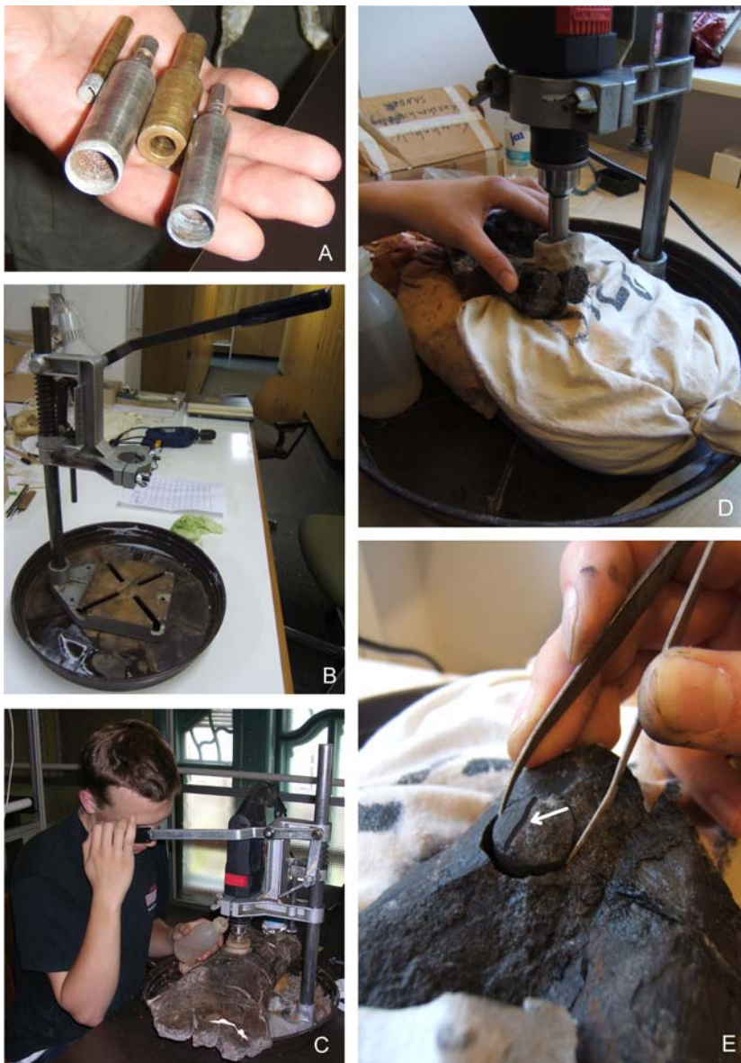
Fig. 9. Histological coring set-up. A: Drill bits. From left to right, 6 mm drill bit, 5/8 inch (15.9 mm) diameter bit, custom-made extension piece for 5/8 inch (15.9 mm) drill bit, and a 1/2 inch (12.7 mm) diameter bit. B: Drill press for normal sized power drill. C: Complete drill set-up. Here a large sauropod humerus is being sampled. Notice the plasticine dam and water being added to cool the drilling site. D: Close-up of the drilling process. Notice that incomplete bones also qualify for sampling, as long as the standard location can be sampled. E: Retrieving the core, after it has been broken from its base with a small screwdriver. Note the mark of the bone long axis on the core, which is important for the correct orientation of the thin section.
