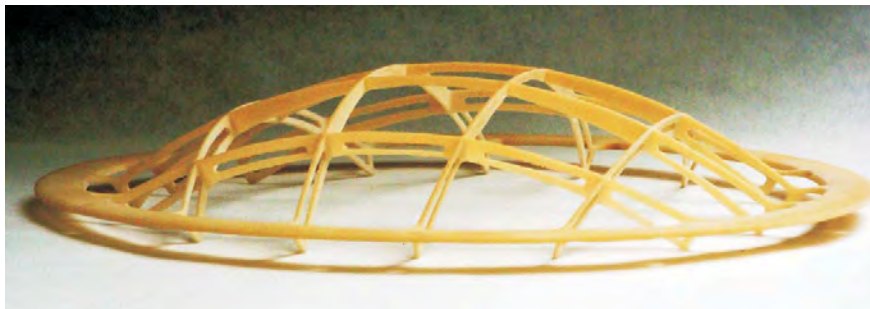
Figure 4.10 — A curved spacer made by stereolithography.
