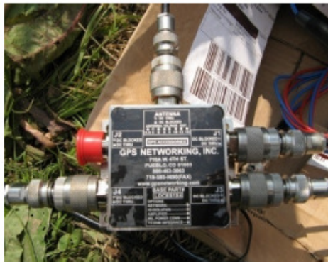
Abb. 5-21: 4-fach Antennensplitter der FIRMA GPS NETWORKING INCORPORATED (2010)
