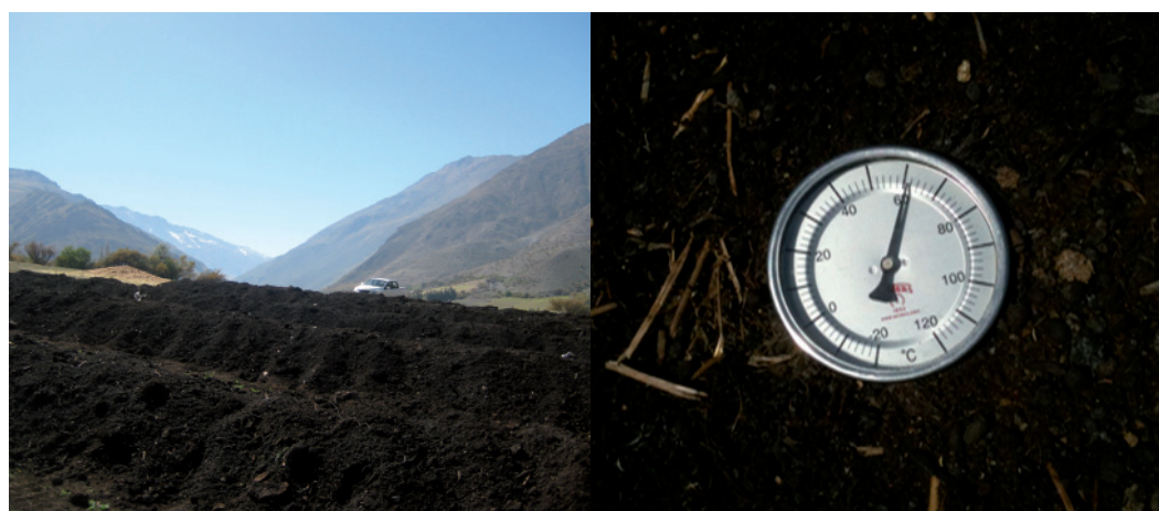
Figure 5.2. a) Compost piles and b) Measurement of the temperature of pile
