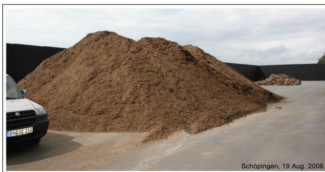
Figure 2.9. Separated solids of digested biogas slurry (Bs) from a biogas plant at Schöppingen, Germany
