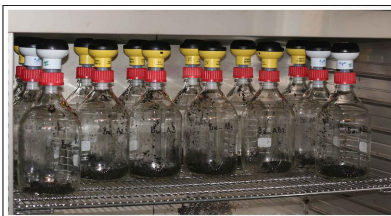
Figure 3.12. Respiration activity for four days (AT 4 ) of measurements on maturity in the incubation cabinet
