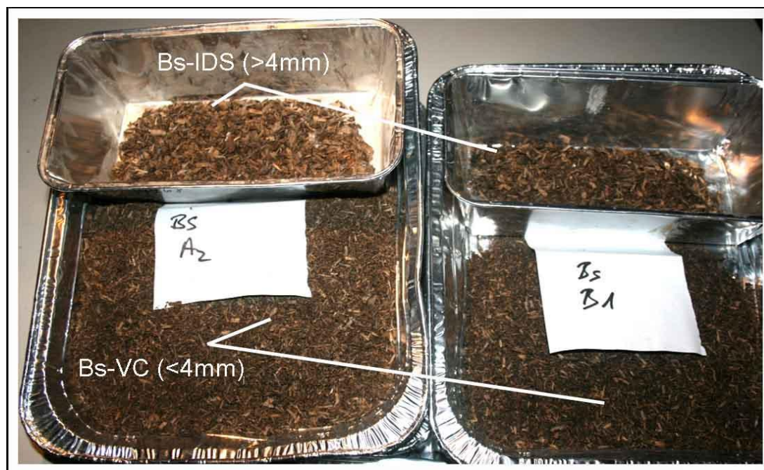
Figure 3.9. Materials sieved into two sizes: the big fraction ( \Phi \geq 4 mm) was named incompletely digested substrate (IDS) and the smaller fraction ( \Phi < 4 mm) vermicompost (VC)
